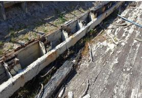
The timber deck and trims shown above are also beyond repair and would need to be replaced around the full boat.
