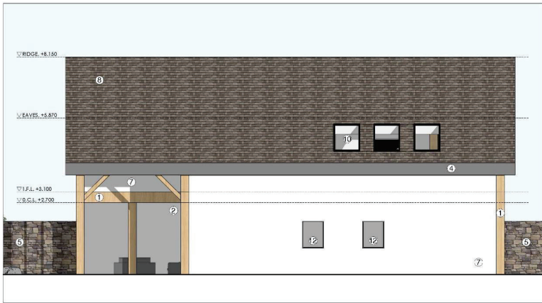
REAR ELEVATION (NORTH-EAST) SCALE 1/80
