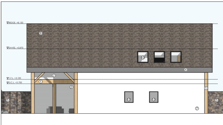
REAR ELEVATION (NORTH-EAST) SCALE 1:50
