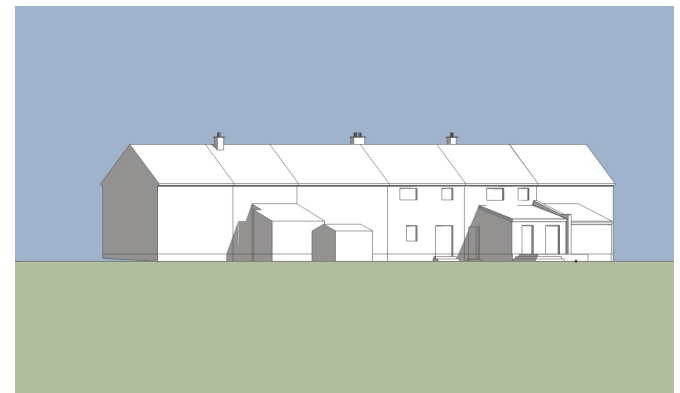
3D Shadow Model - Rear Terrace (South) Elevation View Image taken at Time 09:00am & Date 21 Mar
