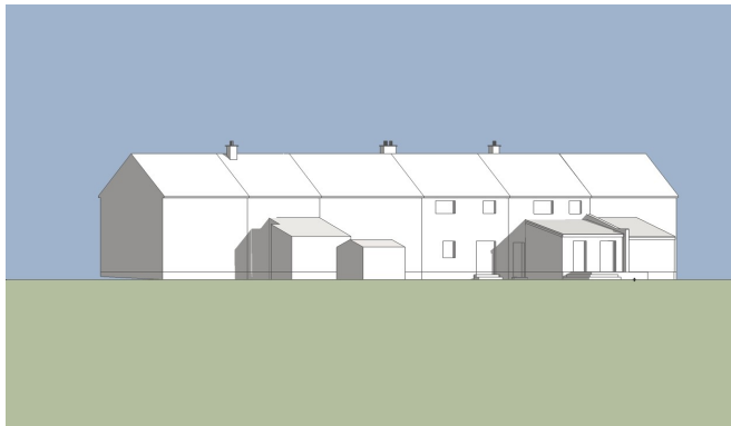
3D Shadow Model - Rear Terrace (South) Elevation View Image taken at Time 08:00am & Date 21 Feb
