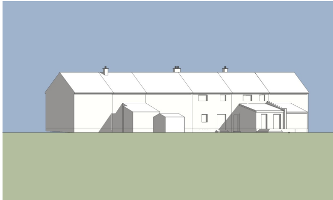
3D Shadow Model - Rear Terrace (South) Elevation View Image taken at Time 08:00am & Date 21 Apr
