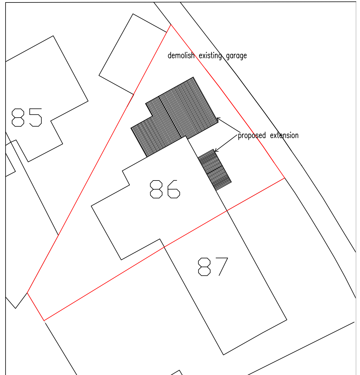
SITE PLAN AS PROPOSED 1:200
