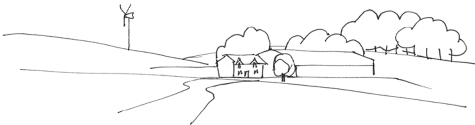
Image 1: Scale in relation to buildings: A turbine illustrated at an indicative 2x the height of the house from this view. The turbine is well scaled in relation to the size of other individual features. It is also located on the side of the hill, rather than the hill top, where it can be 'read' in conjunction with the farm buildings. This forms a 'cluster' of development, which reduces landscape and visual impact.
