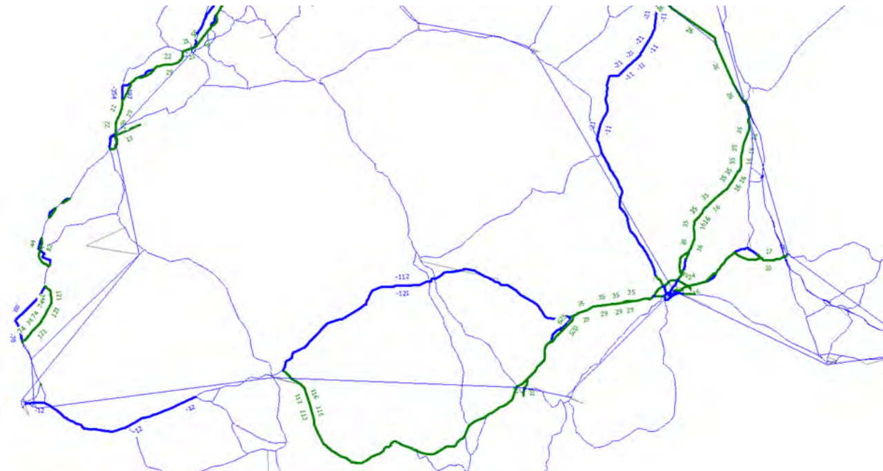
Figure 4-1: Flow difference plot for package 1 minus reference case, AM period, 2045 (total vehicles)
