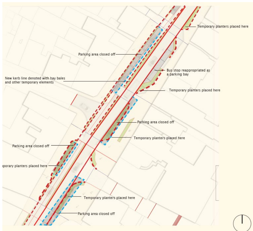
Figure 2.3 - Stage 2 Sandgate Street Trials
